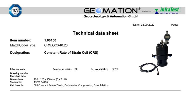
The CRS cell is used to determine the consolidation behavior when lateral expansion is prevented with the help of a constant vertical deformation speed.
